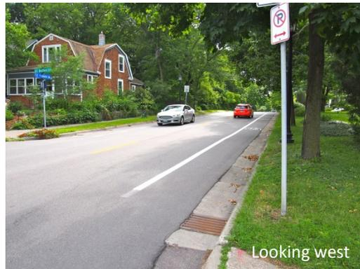
The existing wide and open intersection design allows vehicles to turn onto Bedford St SE at high speeds.
